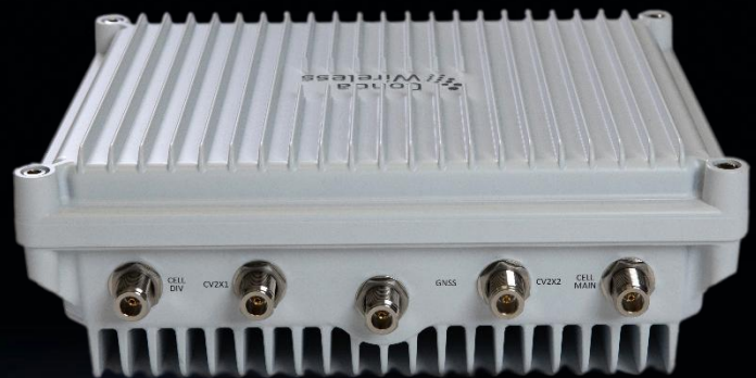
↑ Cellular Diversity ↑ C-V2X 1 ↑ GNSS ↑ C-V2X 2 ↑ Cellular Main
