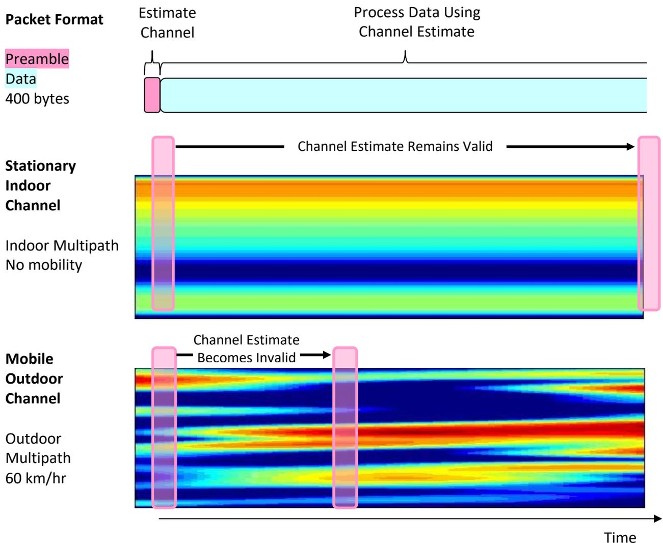
This is what causes the COTS DSRC radios to fail under conditions of simultaneous multipath and mobility. It also explains why the performance of the COTS DSRC radios is worse when the packets are longer – the packets spend more time on the air and channel estimate made during the preamble is more likely to become invalid before the end of the packet.
